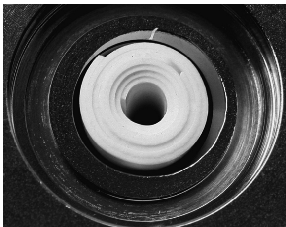
Fig. 4. Membrane M4 wrapped around the frit in a module.
